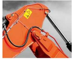
The adaptability to harsh dust work conditions has been improved by increasing the lubrication point of the arm connection unit.
